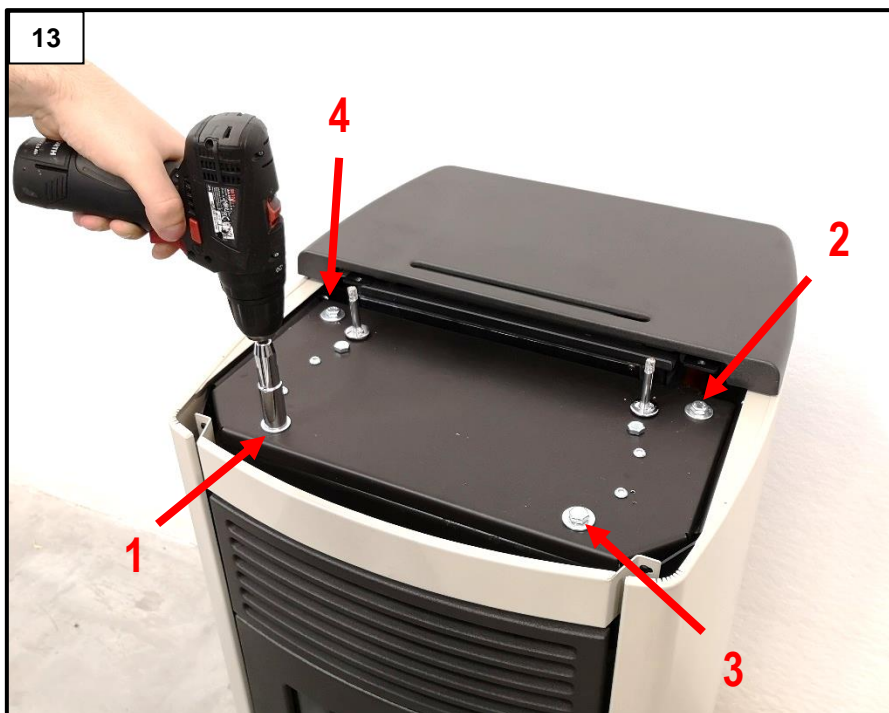
Unscrew the four hex-headed screws, following the sequence given in the photo (Figure 13).
