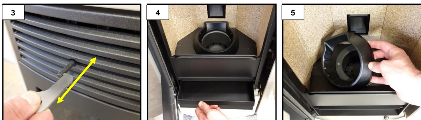
Remove the flame arrester as shown in the diagram (fig. 1 and 2).
